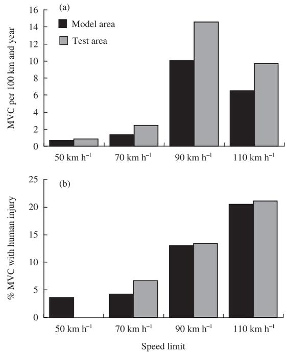
**Fig. 3.** Numbers of moose–vehicle collisions (MVC) per hundred kilometres and year during 1990–99 for different road categories in the model area ( $n = 2185$  MVC) and test area ( $n = 1655$  MVC). (a) MVC densities on roads with different speed limits. (b) Percentage of MVC that involved human injury or death depending on the speed limit of the accident road.
