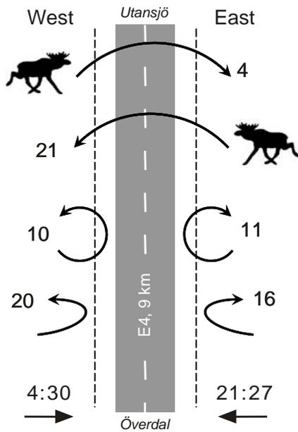
Figure 8. Moose movements along the 9 km section of the new highway E4 during 39 days in first winter after construction and fencing of the road. Snow tracking was done during April, i.e., during a season where migrant moose usually return to their summer home ranges further upland (west).
